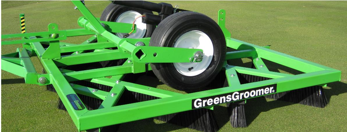
The second generation design increases the effective surface area and improves brush angles which translates into significant performance gains. These changes force topdressing deeper into the canopy, creating a healthier turf system more quickly. The new design also improves the breakup of aeration cores without the need for an additional pass.
